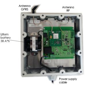
The device features built-in power failure protection — it is powered from a 110/220 VAC mains supply with the option of backup power from lithium batteries, enabling autonomous operation in the event of a temporary power outage
